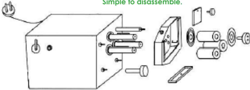
This machine also features an overload protection that will protect the motor in case the machine jams. In the event this does occur, the forward and reverse switch will unjam the unit. The featured gear box reduces the stress on the ½ HP motor, while adding more torque to process even the toughest sugarcane.
