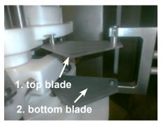
3. Remove the Rosette Blade from the cutout in the connecting unit. Pay attention to positioning and sharp side up. Be sure to lift blade up, by pressing it from the bottom. Then remove it.
