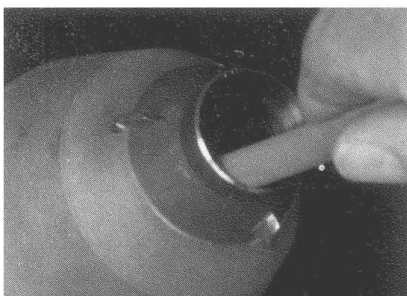
SHARPENING CUTTER WITH WHETSTONE
