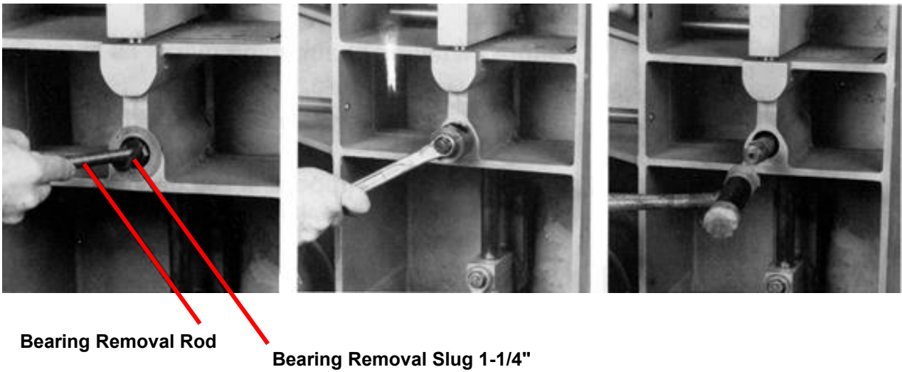
Figure 34. Removing Bearing from Upper Rotary Drive
