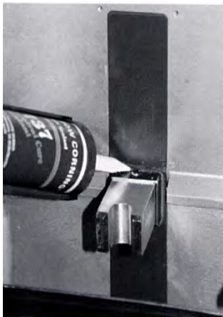
Figure 30a. Installing Lower Splash Guards
