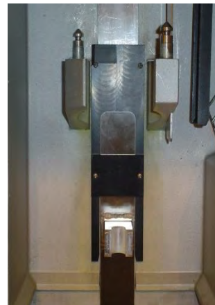
Figure 30b. Installing Center Splash Guard.
