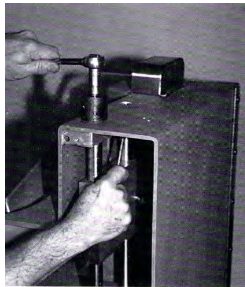
Figure 16. Removal of Linear Shafts with Puller
