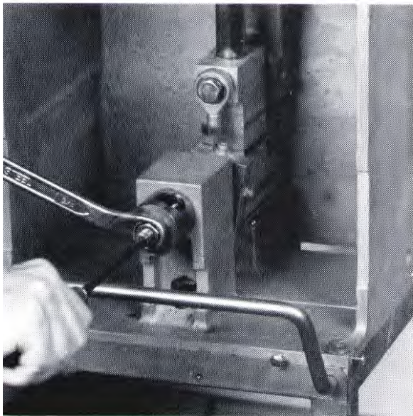
Figure 24. Removing Bearing from Lower Rotary Drive
