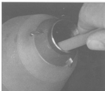
Figure 4a. Sharpening Cutter with Whetstone
